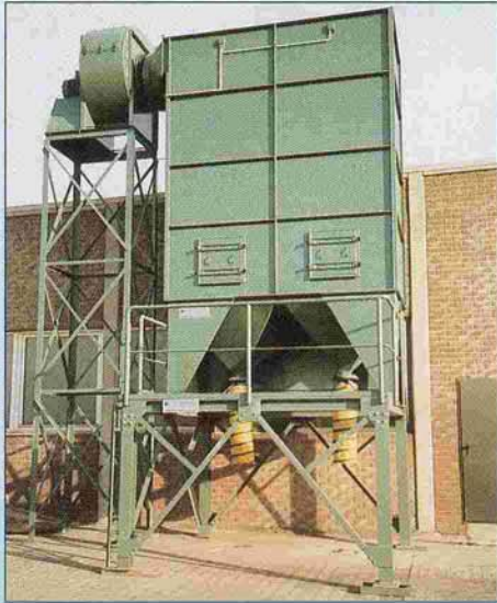
Filter Cobra SMKT-4-150: Cap. 27,000 m 3 /h
