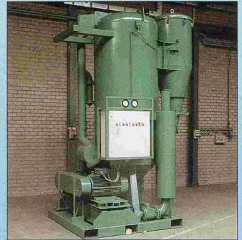
Suction unit with pre-separator
