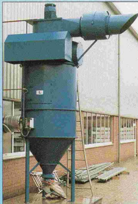
A Pat-Jet 7/13 with built in, centrifugal preliminary separator for extraction fume from a flame cutting machine for aluminium.
