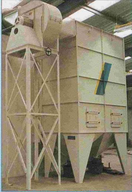
Dust removal by 2 conical flap valves with plastic bag, project Nieuw Amsterdam, Holland.
