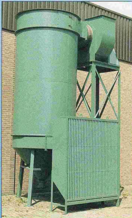
SMT 110 with suction labyrinth, for preservation treatment of trucks, Herten Western Germany.
