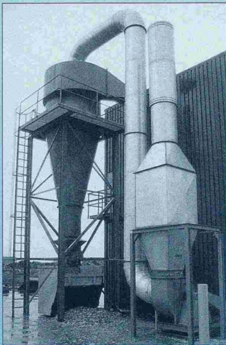
Glasrecycling installation cyclone 2200 mm \varnothing with double chamber air lock, Fan type B 24 \frac{1}{2} , cap. 22,800 m 3 /h, Leeseringen, W. Germany.
