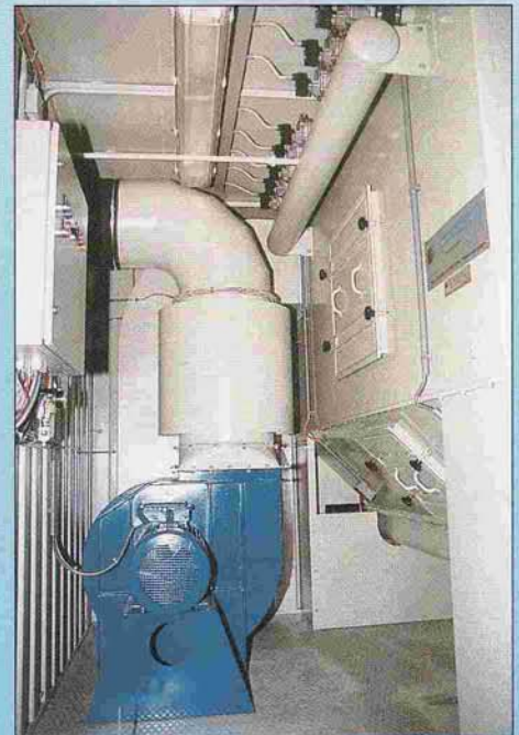
Pat-Jet 16/13 with screw conveyor built in to 10 feet containers, fan B 18 1/4, 11,000 m³/h. Application: suction for outside shot blasting of bridges and chemical plants.
